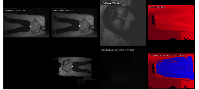
Figure 5. We can simultaneously visualize images from the all sensors alongside debugging information. Note the accurate detection of the bed in the depth field (blue mask).
