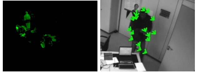
Fig. 3. Left: Foreground segmentation of example input image 2(b) (the higher the distance to the background model the more intense is the green channel); Right: Optical flow extraction for a person entering an office (displacement is magnified for better demonstration)
