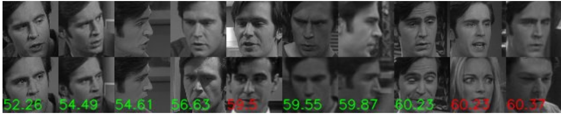
Figure 6.8: Interactive selection of matching faces: The top row shows face images from the query set, the bottom row shows the closest matches from the corpus. The user can select matching face images to assist in the retrieval process.
