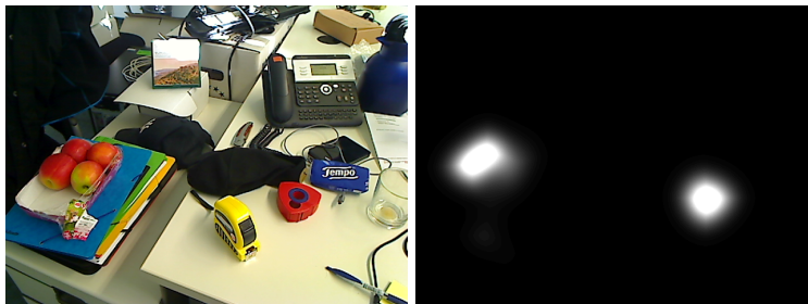
Fig. 1. Illustration of the object detection using color attributes. Image of a typical desktop environment (left) and the corresponding normalized target probability map for color “red” (right). The probability map is calculated at a lower scale than the original image to save computational resources. Here, two potential target objects are clearly identified.
