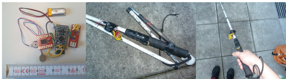
Fig. 2: Left: our haptic module with a battery, arduino processor, bluetooth communication, charger, motor driver, and two linear vibration motors. Total weight: 16g. Center and right: haptic module installed on a white cane with the motors attached to the handle of the cane. The placement of the motors was customizable to each user.
