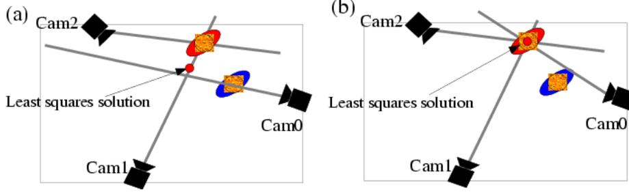
Figure 3. (a) A wrong correspondence (b) A correct correspondence
