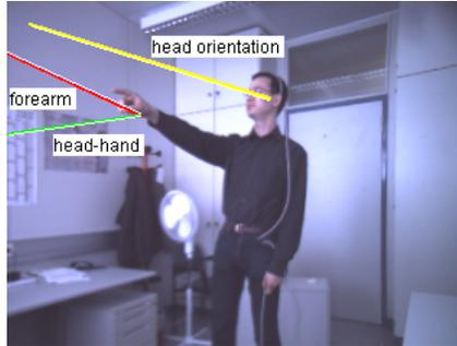
Figure 5: Different approaches for estimating the pointing direction. (The lines were extracted in 3D and projected back to the camera image.)
