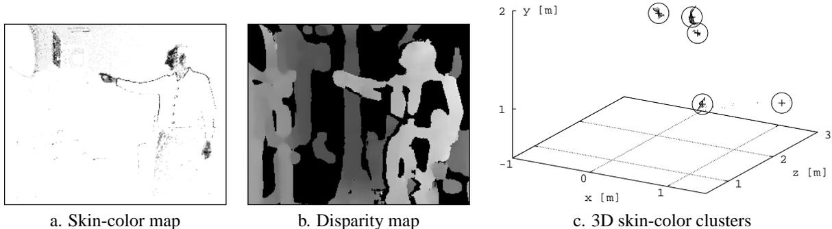
Figure 1: Feature for locating head and hands. In the skin color map, dark pixels represent high skin-color probability. The disparity map is made up of pixel-wise disparity measurements; the brightness of a pixel corresponds to its distance to the camera. Skin-colored 3D-pixels are clustered using a k-means algorithm. The resulting clusters are depicted by circles.
