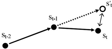
Figure 2: The transition score considers the distance between the predicted position  $s'_t$  and the currently measured position  $s_t$ .
