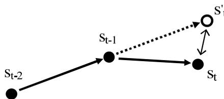
**Fig. 3.** The transition score considers the distance between the predicted position  $s'_t$  and the currently measured position  $s_t$ .
