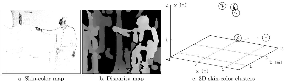
**Fig. 1.** Feature for locating head and hands. In the skin color map, dark pixels represent high skin-color probability. The disparity map is made up of pixel-wise disparity measurements; the brightness of a pixel corresponds to its distance to the camera. Skin-colored 3D-pixels are clustered using a k-means algorithm. The resulting clusters are depicted by circles.
