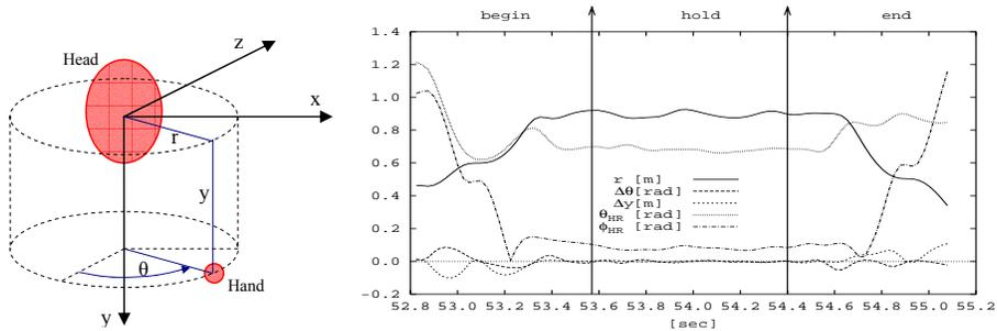
**Fig. 5.** The hand position is transformed into a cylindrical coordinate system. The plot shows the feature sequence of a typical pointing gesture.
