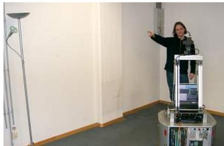
**Fig. 2.** Interaction with the mobile robot. Software components of the robot include: speech recognition, speech synthesis, person and gesture tracking, dialogue management and multimodal fusion of speech and gestures.
