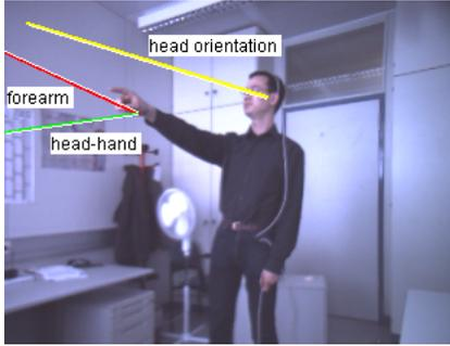
**Fig. 6.** Different approaches for estimating the pointing direction. (The lines were extracted in 3D and projected back to the camera image.)
