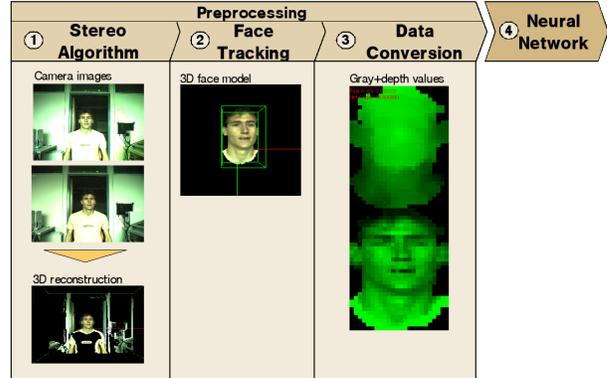
Figure 1: The components of the head pose tracker
