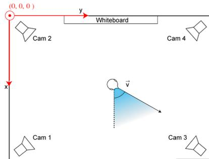
**Fig. 1.** Setup of the CHIL head pose task: four cameras were installed in a room's upper corners to capture the whole area underneath them. This surrounding setup allows people to move and behave without restrictions regarding a specific sensor. Using numerous cameras always guarantees to capture at least one frontal view. However, it is inevitable that some cameras only capture the back of the head, depending on how the head is rotated.
