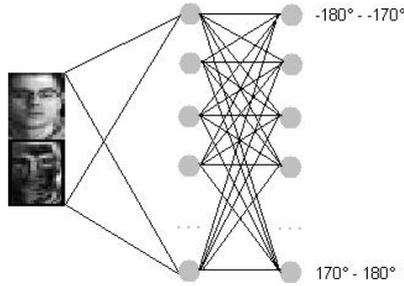
**Fig. 4.** In the multi-view setup, we trained one neural network with 36 output neurons. Each of them represents one discrete head pose class, relative to the camera’s line of view (in  $10^\circ$  steps). The network was trained to estimate the likelihood of a possible rotation, given the observation of that camera.
